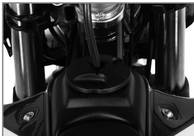
Unscrew the cap to access to the gas tank.
