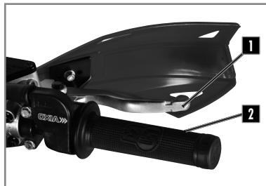
The front brake lever **1** and the throttle twist grip **2** are located on the right side of the handlebar.
