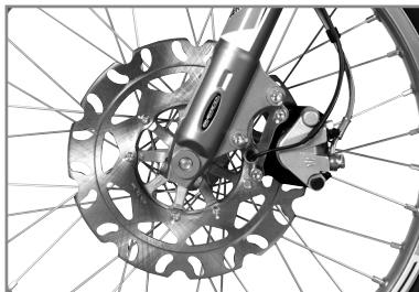
The state of wear of the brake pads can be checked by observing the end of the 2 pads on the caliper (see arrow) they should have a minimum thickness of 2 mm.
