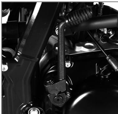
The Kickstarter pedal is located on the right side of the engine. The upper portion rotates.
